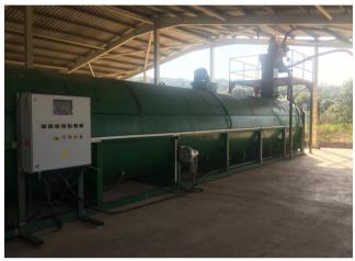
Meet the latest technology <u>Genema Ultra Efficient Composting Bioreactors</u> for organic waste composting! Composting is biological separation and stabilization process of organic wastes (manure, food waste, green waste, abattoir waste etc.) under controlled environmental conditions.
